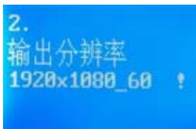
LVP40X has four DVI output ports, i.e.: OUT1, OUT2, OUT3, OUT4, OUT5, OUT6, OUT7, OUT8, each output port has 4 output formats. User can enter item No.2 “*Output Resolution*” to setup it.
