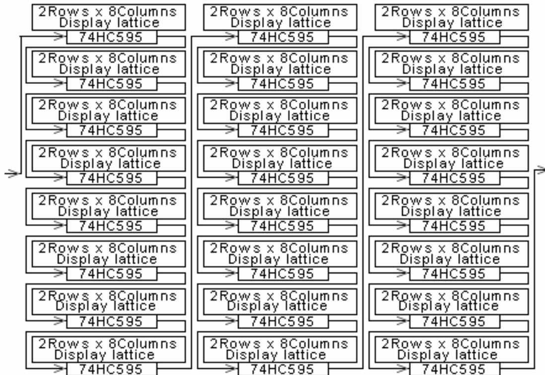
**Mode B: 16 rows/zone:** the signal is shown below; setup method: put the 7<sup>th</sup> switch (1/2) of the receiving card's JP2 on, and keep other switches stay; changing sending card's setup: hardware setup---system setup---row order---reverse per 2 rows, other setups keep default setting.
