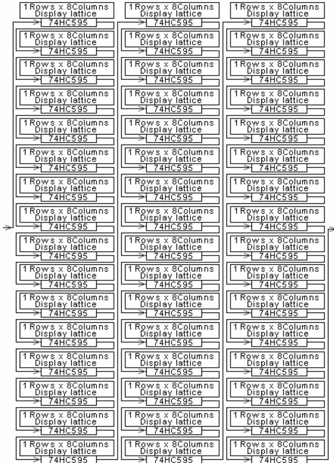
**Mode B: 16 rows/zone:** the signal is shown below; setup method: put the 6<sup>th</sup> and 7<sup>th</sup> switches(1/2) of the receiving card's JP2 on, and keep other switches stay; changing sending card's setup: hardware setup---system setup---row order---all reverse, other setups keep default setting.
