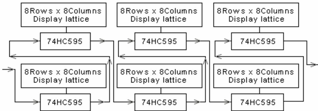
**Mode C: 8 rows/zone:** the signal is shown below; every receiving card can only drive 256 rows height, setup method: the 5<sup>th</sup> switch (1/8) of the receiving card's JP2 is used to select receiving card vertical position, when the switch is "on", the position is upper 256 rows; on the contrary, the position is low 256 rows, and other switches keep stay; changing card's setup: hardware setup---system setup---scanning output---8 rows/zone, and other setups keep stay.
