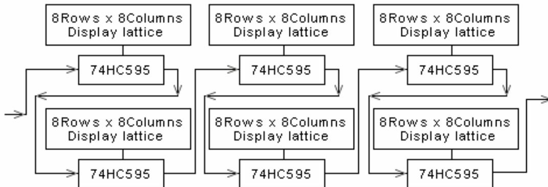
**Mode B: 16 rows/zone:** the signal is shown below; setup method: put the 5<sup>th</sup> switch (1/8) of the receiving card's JP2 on, and keep other switches stay; changing sending card's setup: hardware setup---system setup---row order---reverse per 8 rows, other setups keep default setting.
