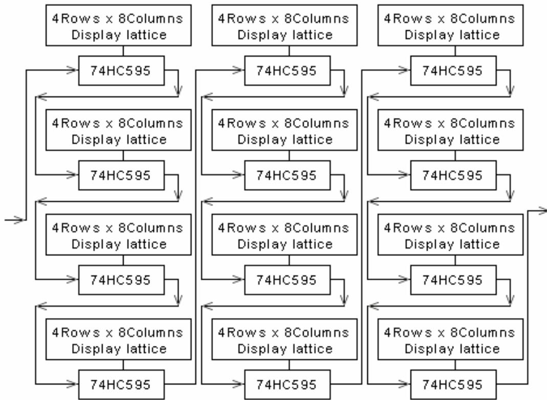
**Mode B: 16 rows/zone:** the signal is shown below; setup method: put the 6<sup>th</sup> switch (1/4) of the receiving card's JP2 on, and keep other switches stay; changing sending card's setup: hardware setup---system setup---row order---reverse per 4 rows, other setups keep default setting.
