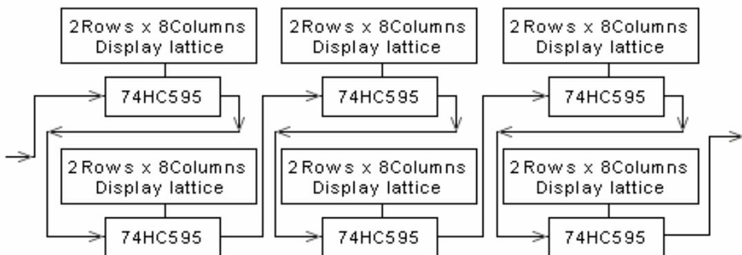
**Mode F 4 rows/zone:** the signal is shown below; every receiving card can only drive 256 rows height, the maximal display is 1024 rows height; setup method: putting the 7<sup>th</sup> switch (1/2) of the receiving card's JP2 on, the 5<sup>th</sup> switch (1/8) of receiving card's JP2 is used to select receiving card vertical position, when the switch is "on", the position is upper 256 rows; on the contrary, the position is low 256 rows, and other switches keep stay.
